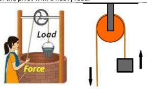
**Pulleys** have a rope or cable which goes over a wheel. This is pulled to lift, lower or move heavy objects.
